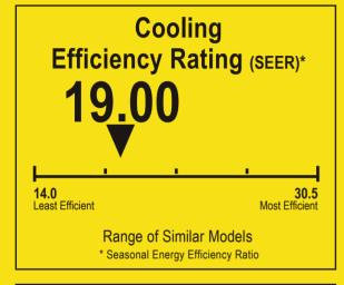
This system's efficiency ratings depend on the coil your contractor installs with this unit. The heating efficiency rating varies slightly in different geographic regions. Ask your contractor for details.
